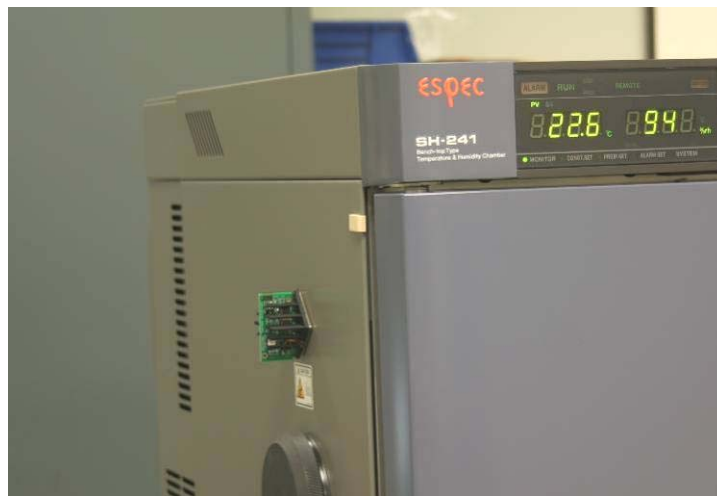
Figure 6: WPG-1 mounted vertically on side of oven using adhesive
